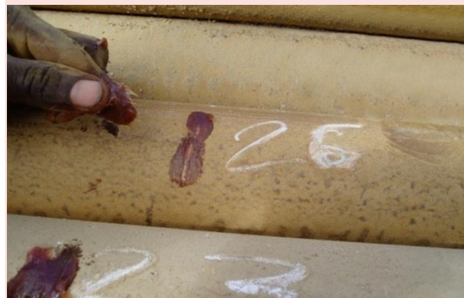
Figure (above) Drill-rod marking so that samples, penetration rates and air-lift yield can be accurately recorded
