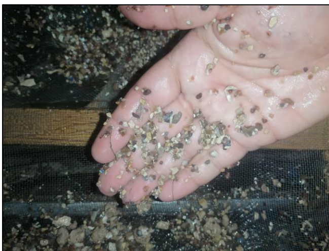
Figure 6: Samples are laid out and logged for 1m depth intervals
